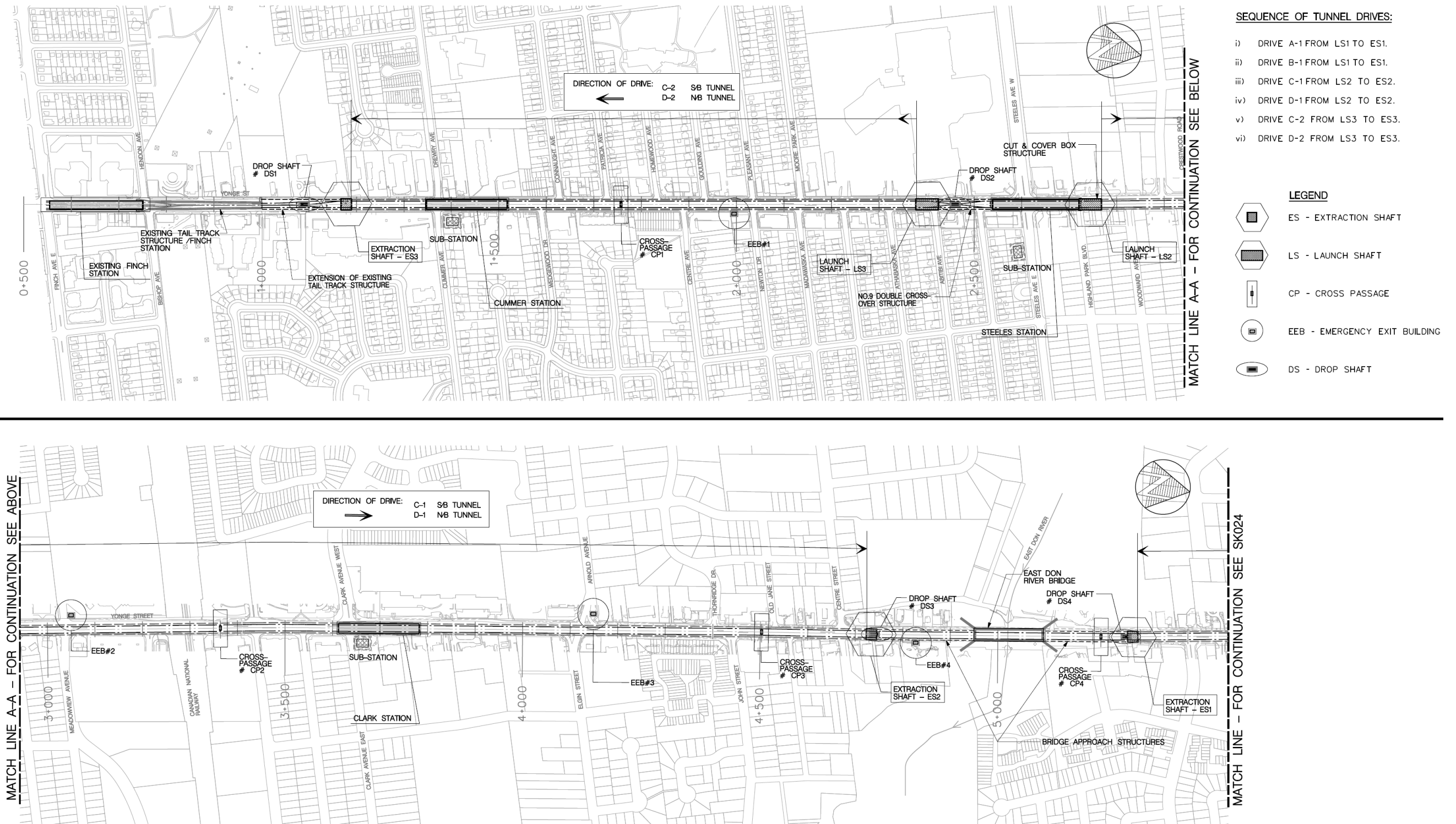
Figure 14-1: Proposed Tunnelling General Arrangement (Finch Station to North of the East Don River Bridge)
