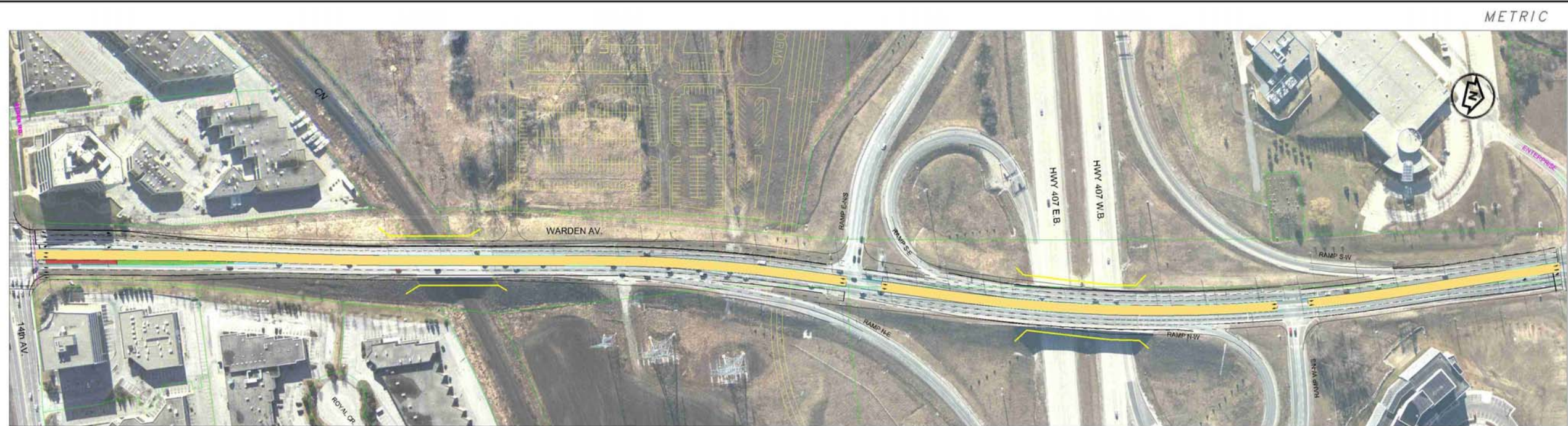
ALTERNATIVE B1 - Median Transitway plus 6 traffic lanes
