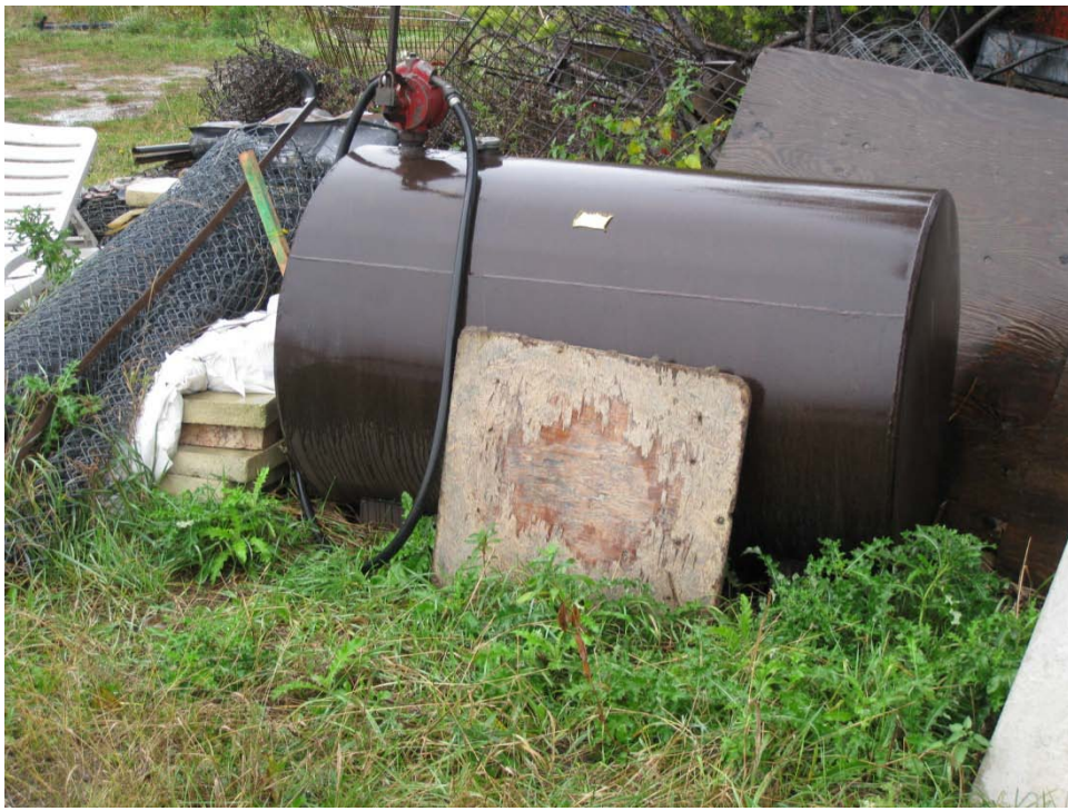
Photograph 3: View of the diesel AST observed in the Rosa & Maria Farms.
